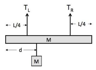
A beam of mass M=4.3 kg and length L=5.1 m is suspended by two vertical ropes as shown. The rope on the left has tension  $T_L$  and is attached a distance L/4 from the left end of the beam. The rope on the right has tension  $T_R$  and is attached a distance L/4 from the right end of the beam. A box that has the same mass M as the beam is suspended by a short rope which it attached a distance d from the left end of the beam.
