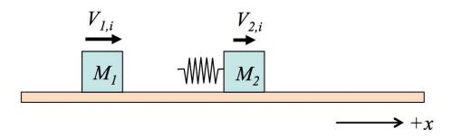
A block of mass  $M_1 = 2$  kg is moving to the right with initial speed  $V_{1,i} = 3.4$  m/s. It collides with another block of mass  $M_2 = 3$  kg that is initially moving to the <u>right</u> with  $V_{2,i} = 1.7$  m/s. There is a massless spring connected to the second block as shown, and the collision between the blocks is elastic. All motion is in one dimension and the +x direction is to the right in the picture.
