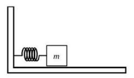
A mass m = 3 kg is placed on an ideal spring with spring constant k = 185 N/m and is free to oscillate on a horizontal surface with no friction. The mass is pulled 16 cm to the left of equilibrium and released at t = 0.
