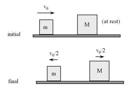
A box of mass m slides on a frictionless horizontal air-track with an initial speed  $V_0$ . It collides and bounces off a box of mass M which is initially at rest. After the collision the boxes have the same speed,  $V_0/2$ , one moving to the left and the other to the right as shown.
