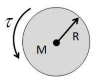
A uniform solid cylinder having mass M=2.4~kg and radius R=0.43~m is free to rotate around a fixed frictionless axle through its center (out of the page in the figure). The cylinder is initially at rest and at t=0 a constant torque with magnitude  $|\tau|=9.763~Nm$  is applied around the axis causing the cylinder to rotate.
