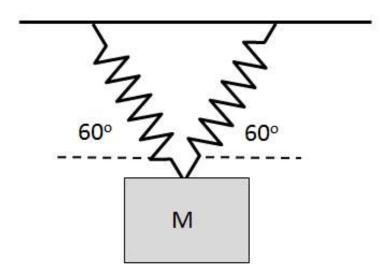
A mass, M=3.2 kg, hangs motionless from the ceiling from two identical ideal, massless, springs with spring constants k=507 N/M. Each spring makes an angle of  $\theta=60^o$  with respect to horizontal as shown.
