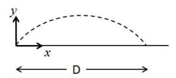
A ball is launched from ground level and hits the ground again after an elapsed time of 4 seconds and after traveling a horizontal distance of 56 m. The only force acting on the ball is gravity.
