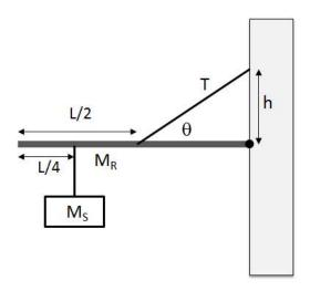
A horizontal rod of length L and mass  $M_R = 1.8$  kg is used to hang a sign on a wall. The right end of the rod is attached to the wall by a hinge. A wire having tension T runs from the center of the rod to a place on the wall a distance h above the hinge as shown. The wire makes an angle  $\theta = 28^{\circ}$  with the rod. The sign has mass  $M_S = 0.6$  kg and hangs distance L/4 from the end of the rod. The system is in equilibrium.
