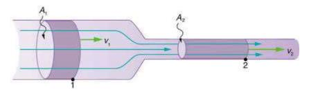
An incompressible fluid (density 1000 kg/m³) flows through a horizontal pipe with cross sectional area  $A_1 = 0.0045 \text{ m}^2$  and speed  $v_1 = 3.2 \text{ m/s}$ . The pipe tapers down to a cross sectional area of  $A_2 = 0.0019 \text{ m}^2$ .
