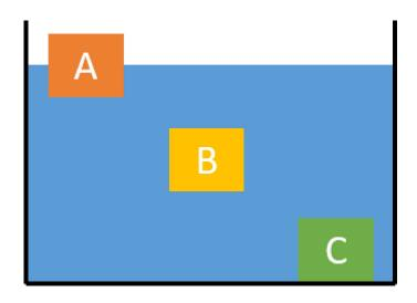
Three masses are in a swimming pool filled with water (density  $1000 \text{ kg/m}^3$ ). All three objects are identical in size ( $400 \text{ cm}^3$ ) but have different densities. Object A floats on the water (density  $580 \text{ kg/m}^3$ ), Object B is completely submerged underwater but has a density equal to that of water, and Object C sinks to the bottom (density  $3700 \text{ kg/m}^3$ ).
