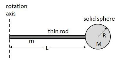
A uniform solid sphere having mass M and radius R is attached to the end of a uniform thin rod of length L and mass m. The moments of inertia of a rod and of a sphere are given in your formula sheet.
