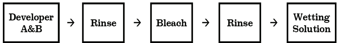
Figure A.1: Hologram processing chain with the JD-2 developer.
