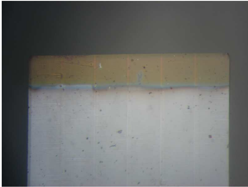
Figure D.1: Photo taken under a microscope of the end of a damaged PPLN crystal. The discoloration of the first \sim 1 mm is evident.
