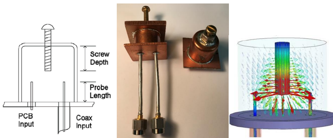
Figure C.3. Conceptual side-view (left), actual implementation (middle), and EM simulation (right) of 10 GHz bandpass pipe cap filters designed for filtering the high-speed WTDC clock. The tuning screw sets the quarter-wave resonance and is capacitively coupled to the input probes. Figures courtesy of [124].
