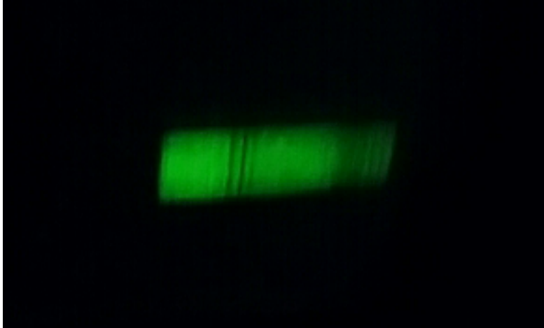
Figure 1.5: First diffracted order of a diffraction grating when illuminated by the expanded HeNe laser at \lambda = 532\text{nm} of the Diffractometer, showing obvious variation in efficiency. Visible streaks are common in mechanically ruled gratings.
